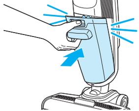
**12.** Reinstall dirty water tank. Insert bottom of tank first. Pivot top toward the machine until it clicks into place.
