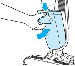
**4.** Press button on top of dirty water tank. Grip front handle and pull out to remove.
