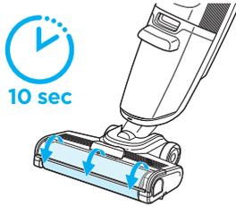
**5.** Brush roll starts spinning. Brush roll will not spin when machine is upright. The solution may take up to 10 seconds to fully wet brush roll.
