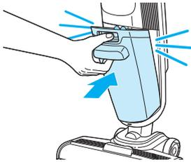
**7.** Insert bottom of tank first. Pivot top toward the machine until it clicks.
