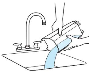
**5.** Pour dirty water into a sink or similar wastewater receptacle and thoroughly rinse tank.
