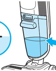
**1.** Empty dirty water tank when water reaches "MAX" line. Do not let water overflow.
