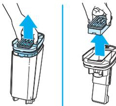
**5.** Pull up tank lid to remove filter assembly. Grip sides of filter to remove filter.
